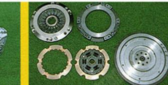
This is the equiped twin plate ceramic metal clutch. The total weight of the clutch system is 10% lighter than stock, and the inertia mass is reduced by about 15%, improving the response and feel.
