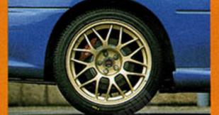
On the rear are 15" rear ventilated rotors with 2 pot calipers. Both the front and rear calipers are painted in red to appeal to the potential of the 22B STi. However, the part itself is the same as the convential STi.
