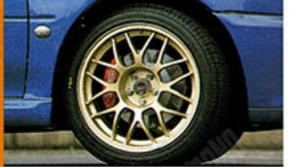
The tires are Pirelli P-Zero (235/40ZR17). The forged 8.5x17+48 offset"BBS wheels weigh the same as the OEM 16" wheels! Due to the hub change and offset, the track is 10mm wider in the front and 40mm in the rear.
