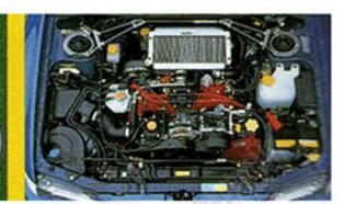
The 2212cc EJ22 puts out 280PS/ 37.0kgm. The intake manifold is painted with wrinkle red paint, like the standard STI version, but unique to the 22B are the wrinklered-painted timing belt covers.
